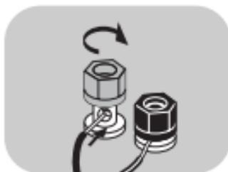
Using the five-way binding posts: The binding posts permit easy connection to banana plugs, spade lugs, and bare wire. Insert the wire in the hole and tighten.
